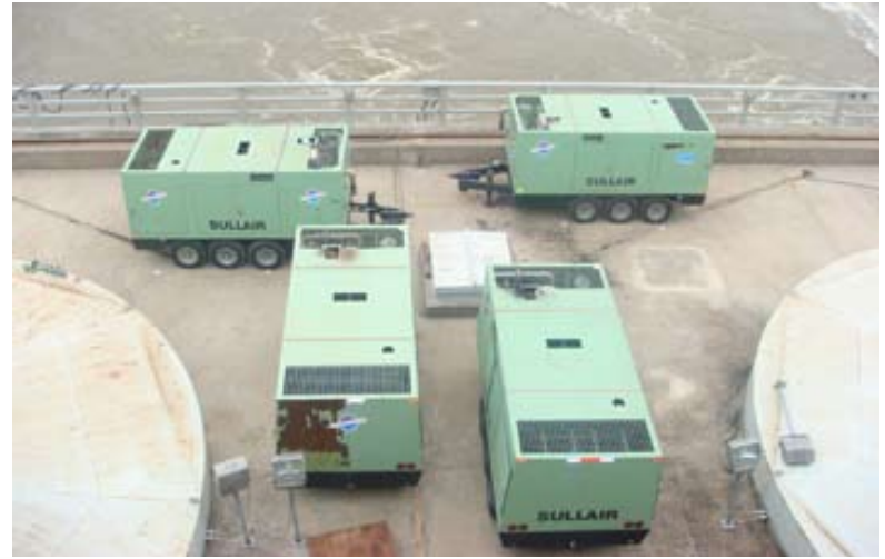
GRDA crews and contractors unload air compressors to be used for forced air testing procedures at GRDA's Robert S. Kerr Dam.
