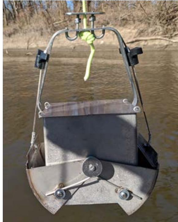
Figure 28 Ekman Dredge Used for In-Channel Sediment Sampling
