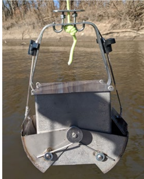
Figure 28 Ekman Dredge Used for In-Channel Sediment Sampling
