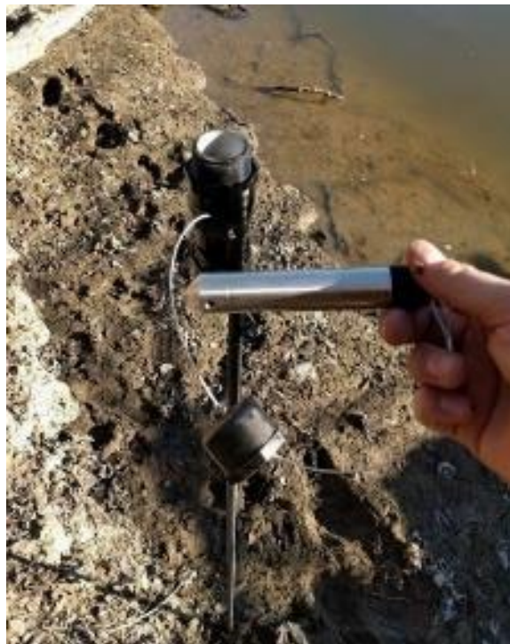
Figure 26 Photograph of HOBO Pressure Loggers and Mounting Chamber
