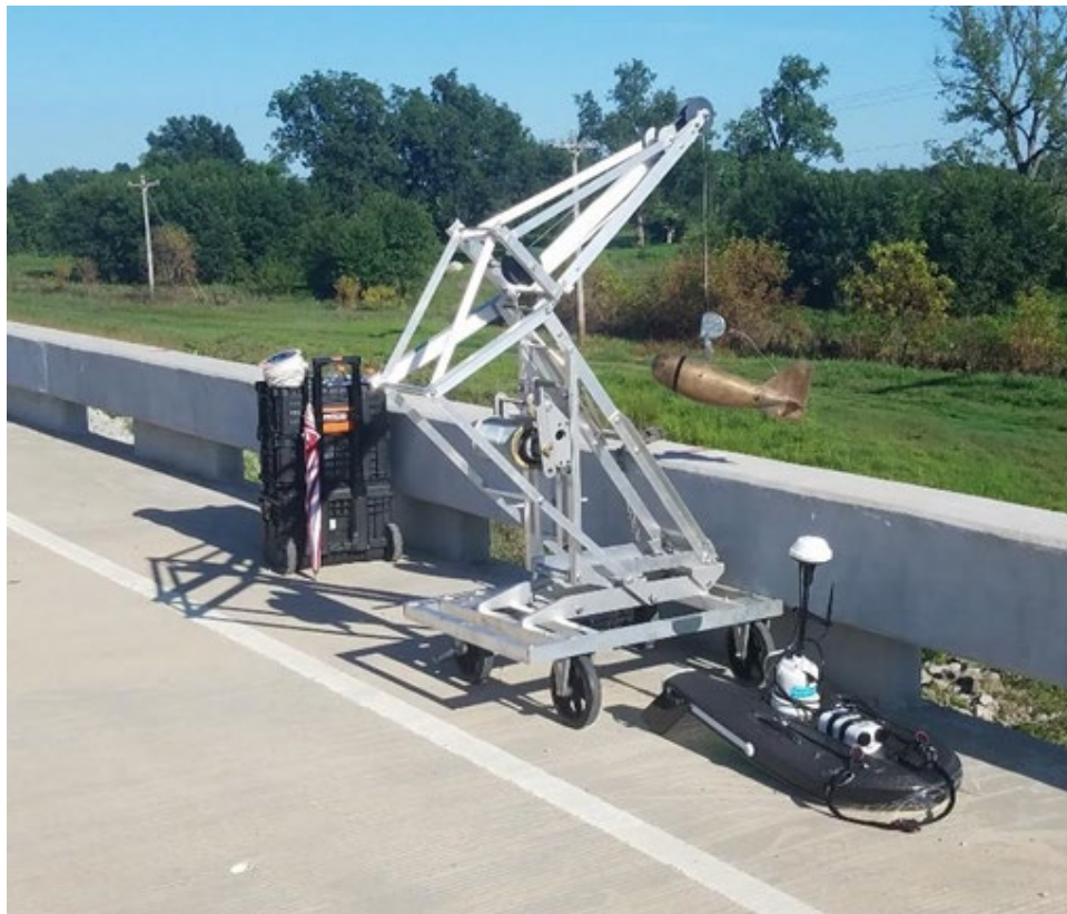
Figure 32 Sampling Equipment Used During Suspended Sediment Concentration Sampling Efforts
