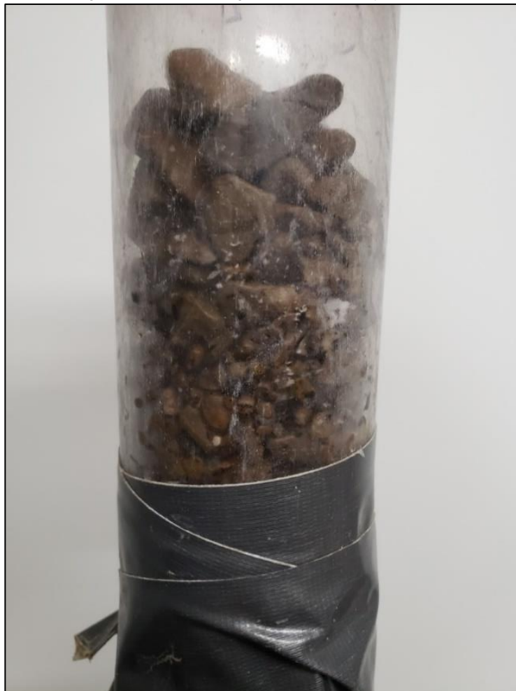
Figure 3.3.1.7.6-8 Sample Image of Core 4 Showing Natural Armor Layer at Bed Surface and Finer Material Below
