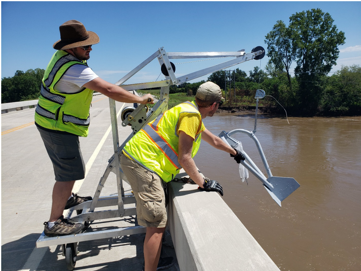
Figure 33 Bedload Transport Measurements Collected Using the Helley-Smith Sampler
