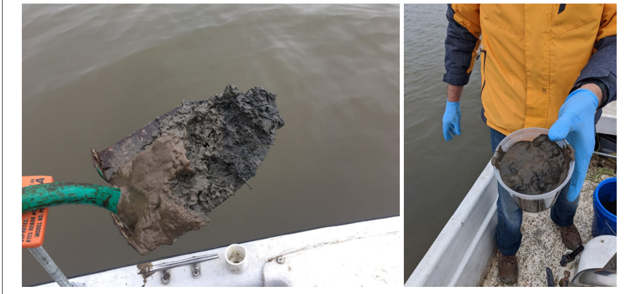
Figure 38 Sediment Grab Samples Collected from the Reservoir Bed in Grand Lake
