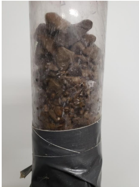
Figure 3.3.1.7.6-8 Sample Image of Core 4 Showing the Natural Armor Layer at the Bed Surface and Finer Material Below
