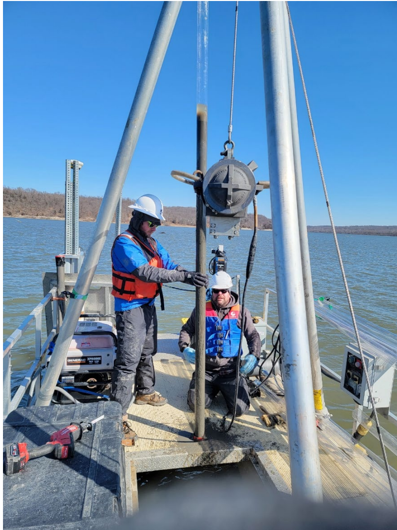
Figure 3 Vibracore System Used during February 2022 Sample Collection
