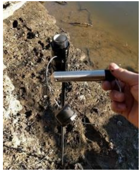
Figure 2 HOBO water level logger prior to deployment
