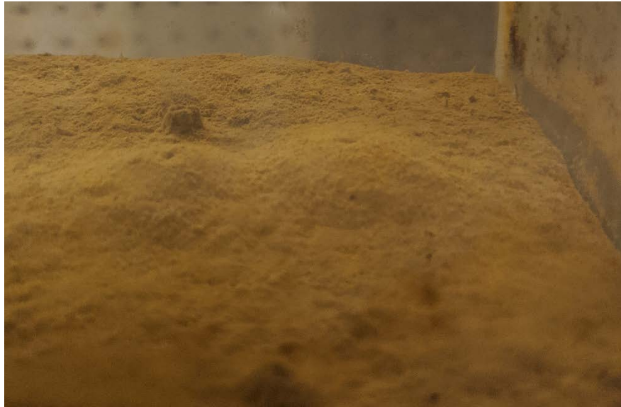
Figure 39. Evidence of biotic activity on surface of SR-TB
