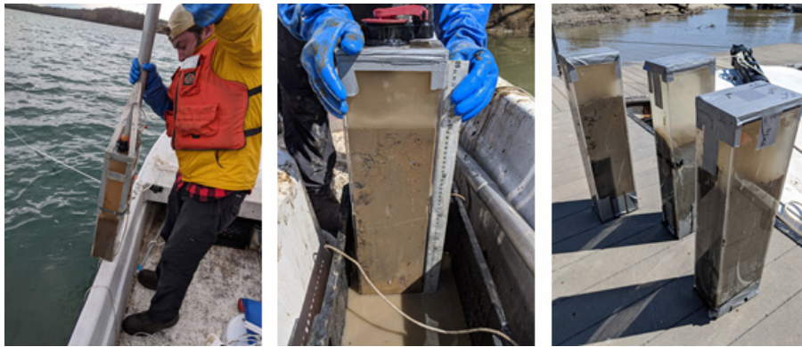
Figure 30 SEDflume Core Sampling
