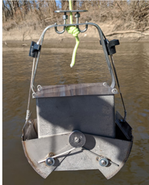
Figure 28 Ekman Dredge Used for In-Channel Sediment Sampling
