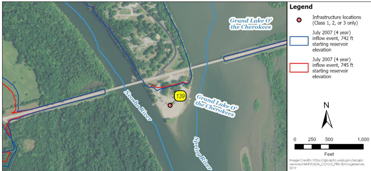
Figure 10. July 2007 event inundation at Twin Bridges State Park (ID 139).
