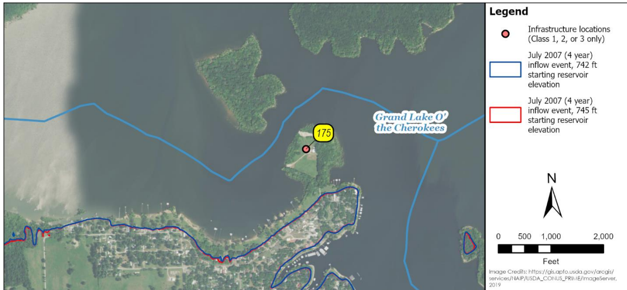
Figure 15. July 2007 event inundation at Cherokee Seaplane Base (ID 175).
