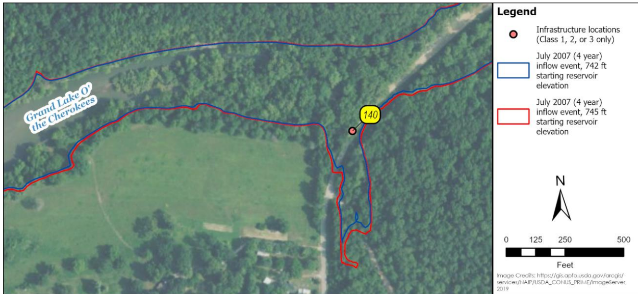
Figure 11. July 2007 event inundation at Shawnee Branch Bridge (ID 140).
