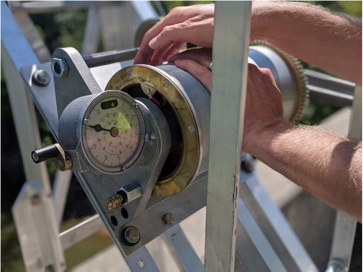
Figure 22 Gage on Winch Used to Determine Length of Cable Let Out during Sampling
