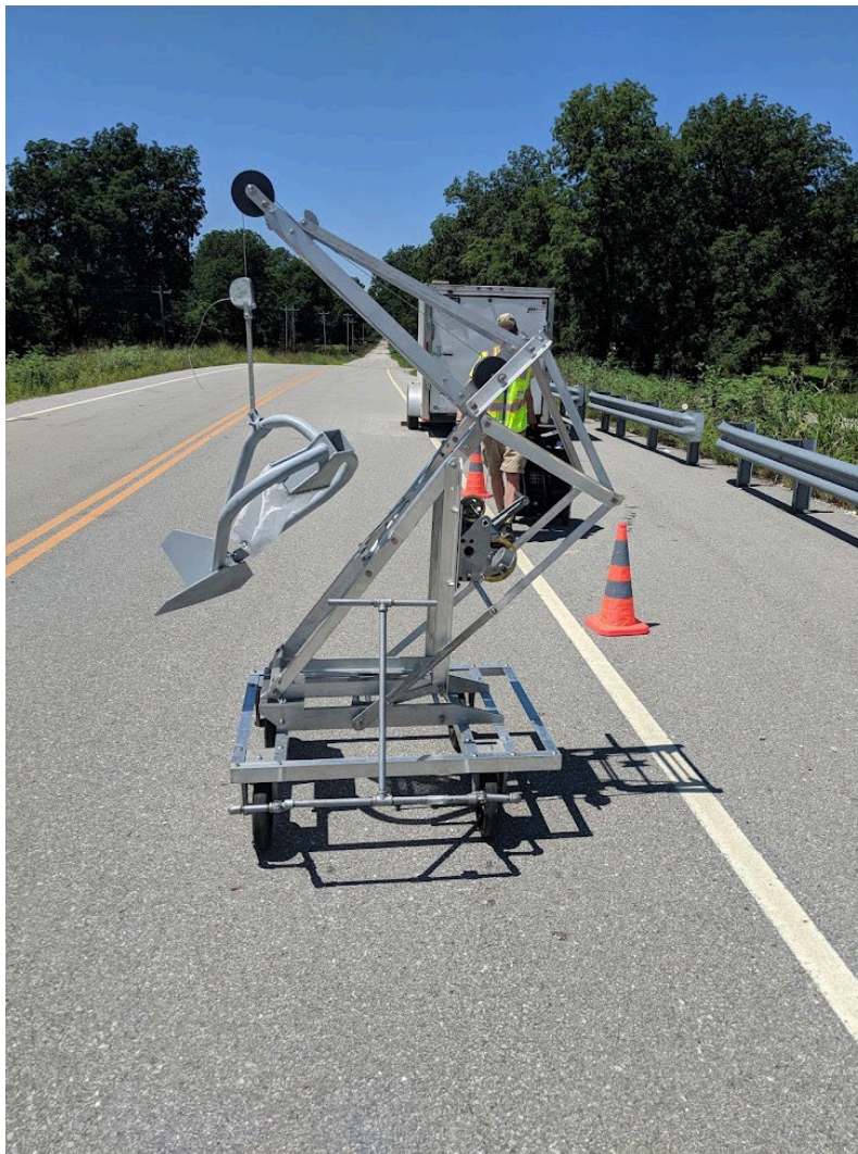
Figure 18 Bedload Transport Measurements Collected Using the Helley-Smith Sampler
