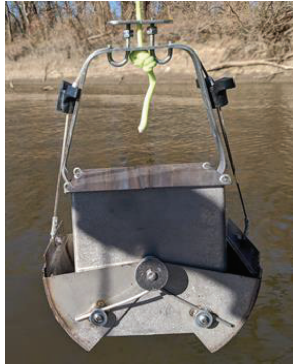
Figure 7 Ekman Dredge Used for In-Channel Sediment Sampling
