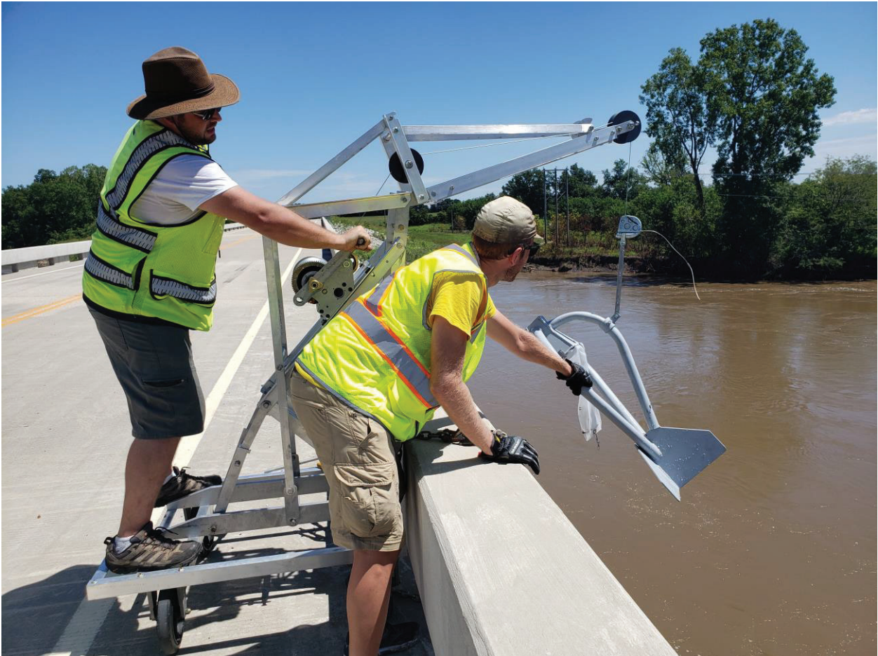
Figure 12 Bedload Transport Measurements Collected Using the Helley-Smith Sampler
