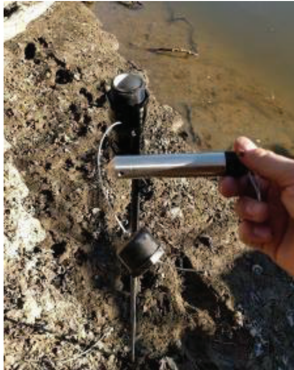
Figure 5 Photograph of HOBO Pressure Loggers and Mounting Chamber
